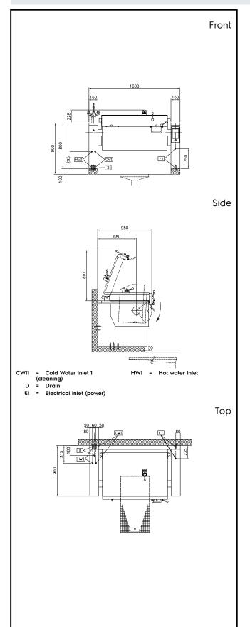
**Electric** Supply voltage: 400 V/3N ph/50/60 Hz Total Watts: 20.6 kW Installation: FS on concrete base;FS on feet;On base;Standing Type of installation:
